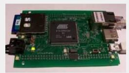
The Linuxstamp is an open source processor module based on the Atmel AT91RM9200 processor. All development can be done with the USB device port which is connected (via USB/serial chip) to the debug serial port on the Linuxstamp. The board's processor, a 180 MHz Atmel AT91RM9200 system-on-chip, integrates an ARM9 CPU core (with MMU) along with controllers for USB host and device ports, 10/100 Ethernet, MMC/SD card interface,
